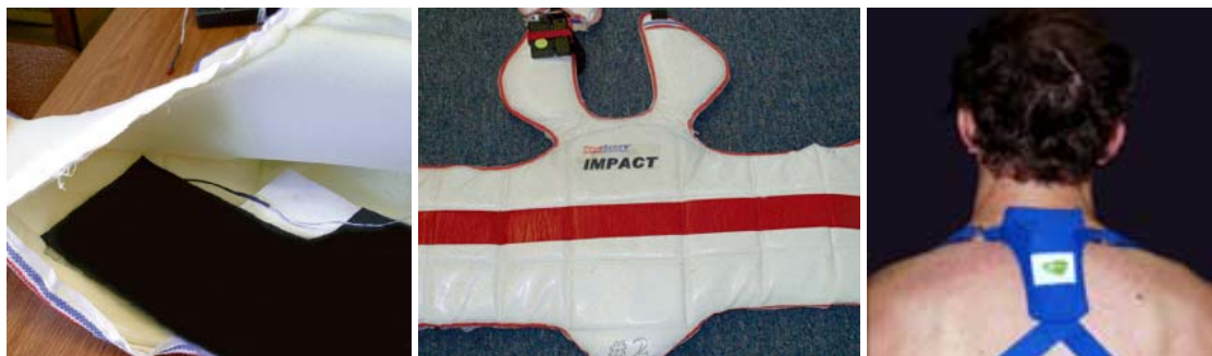
Figure 2.6. Force sensors integrated into Tae Kwan Do protective padding (Chi et al., 2004) (left); wearable GPS technology fitted to AFL athletes (White, 2005) (right).
