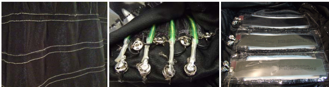
Figure 5.3. Vinyl pockets for panel displays (left) and wire displays, also showing press studs (middle); conductive thread sewn into jersey fabric (right).
