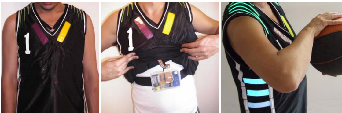
Figure 4.9. Final TeamAwear prototype (left); showing wearable computer connection and harness worn underneath the jersey (middle); final prototype during use (right).
