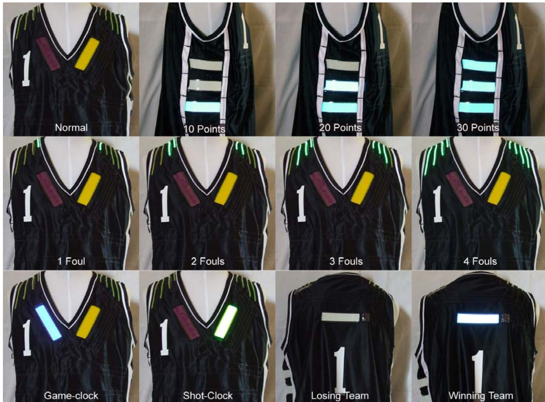
Figure 4.10. The final information sources displayed on the TeamAwear jersey during use.
