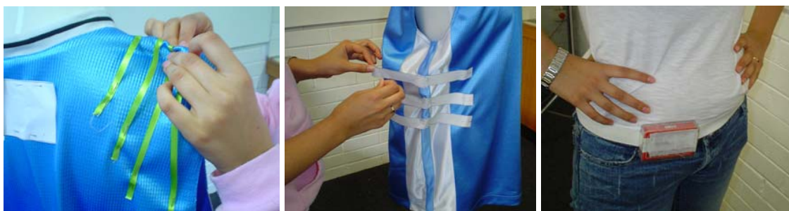
Figure 4.6. Hands-on physical design to determine display locations (left and middle); determining appropriate positioning of wearable computing box (right).
