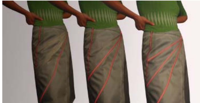
Figure 2.11. The HearWear display varying from quite to noisy environment (Iossifova and Kim, 2004).
