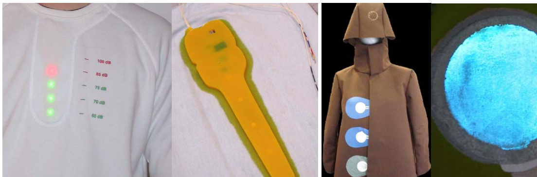
Figure 2.12. The noise shirt with washable coating for electronics (Iso-Ketola et al., 2005) (left); the Glow luminescent raincoat system (Co, 2001).
