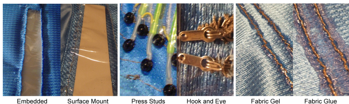
Figure 4.7. Different integration methods tested: display attachment (left); Connecting displays (middle); sealing electric connections (right)
